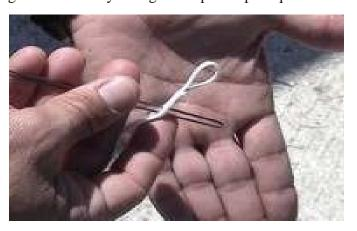
loading or density altitude. Locate the toggle mark on the control line. Insert the finger trap tool beyond this mark, far enough away to accept the running end inside the line and exit at the mark. Make a loop with approximately 2" circumference and fingertrap. The idea is to use the width of the toggle as a measuring guide for the size of the loop.It should be just long enough to go around or over the toggle.
